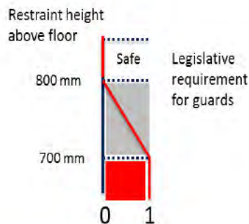
Figure 34_14: Illustration of safe, grey and red zones for height of restraint assessment
